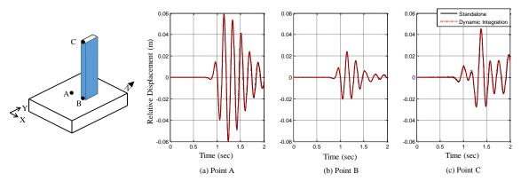
Figure 6. Verification of the proposed dynamic integration framework against the standalone analysis at three points.
