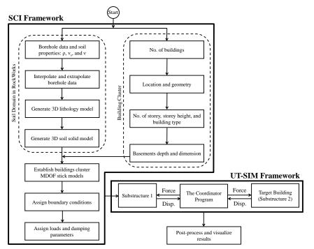
Figure 1. Procedure of the development of the multi-scale SCI framework.
