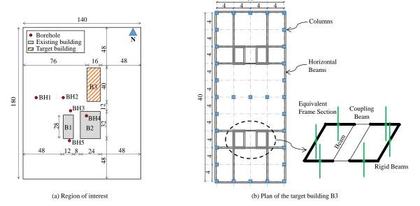
Figure 2. Region of interest and the target building (all units are in m).
