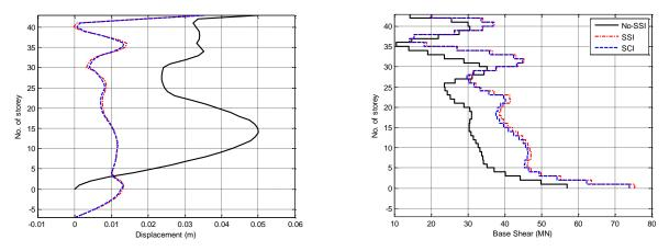
Figure 7. Peak lateral displacement and base shear force distribution along the height of building B3.
