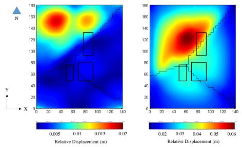
Figure 4. Distribution of the free-field peak ground displacement, at surface, along the X-direction (left) and the Y-direction (right) (the black boxes indicate the location of the buildings).
